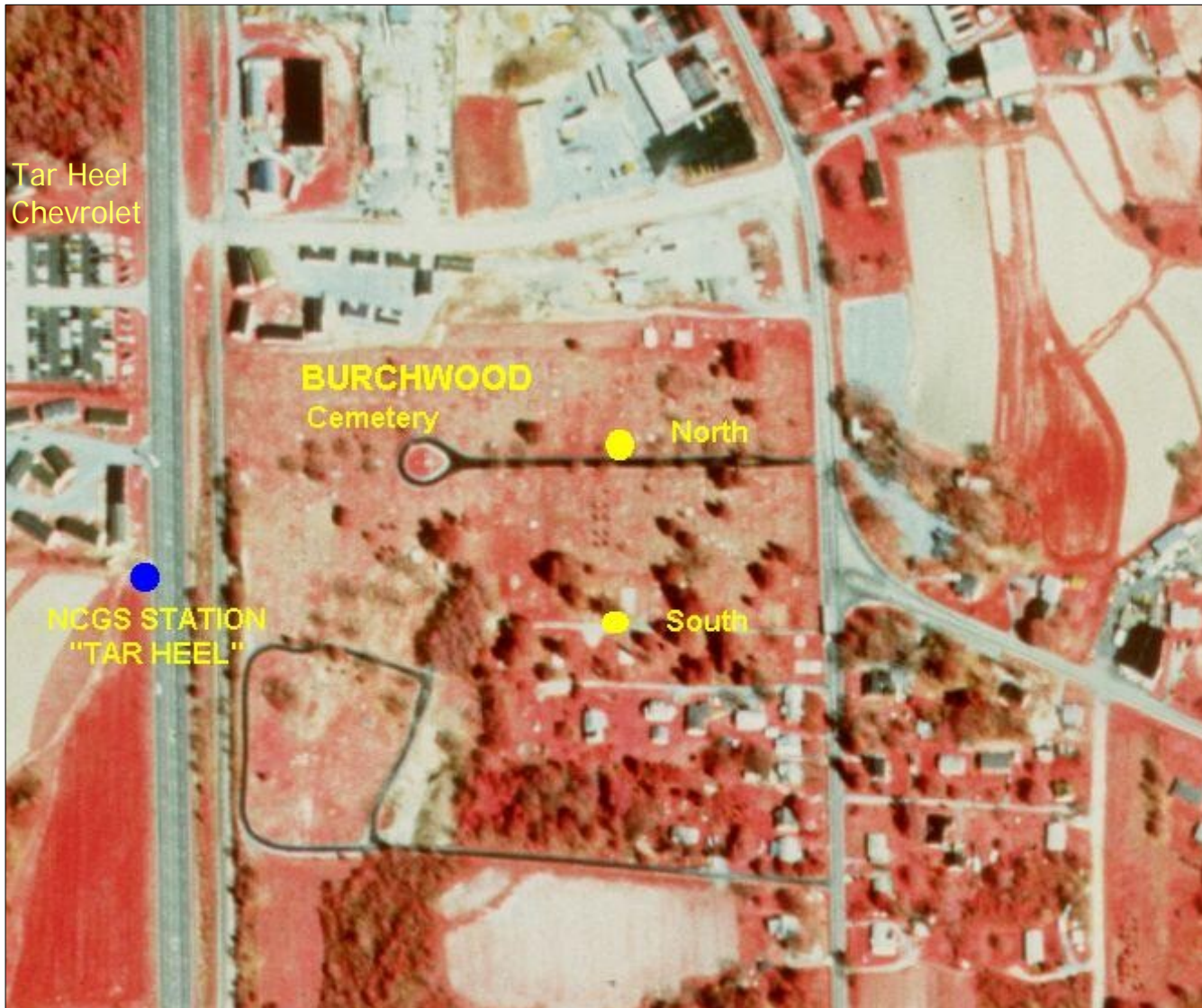
Figure 3. An infrared aerial photo of the Burchwood Cemetery, which is located south of Roxboro in Person County, showing the location of the north and south meridian monuments, the Tar Heel Chevrolet dealership, and NCGS station TAR HEEL (FY1854).
